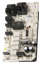
Main Control Board
