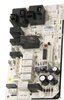
Main Control Board
