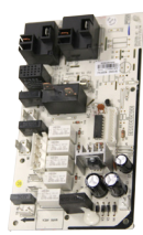
Main Control Board
