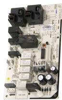
Main Control Board
