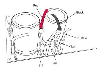
8. Locate the Rectifier on the rear wall of the unit.
