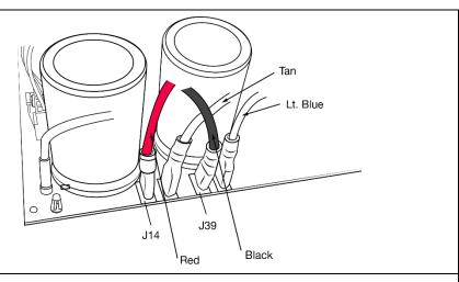
6. To remove Terminal Plugs, and prevent damage to the board, make sure to press the release lever.
