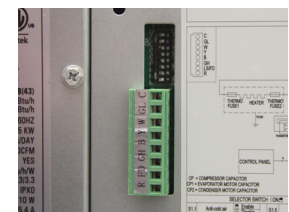
Energy Management & Thermostat Connections
